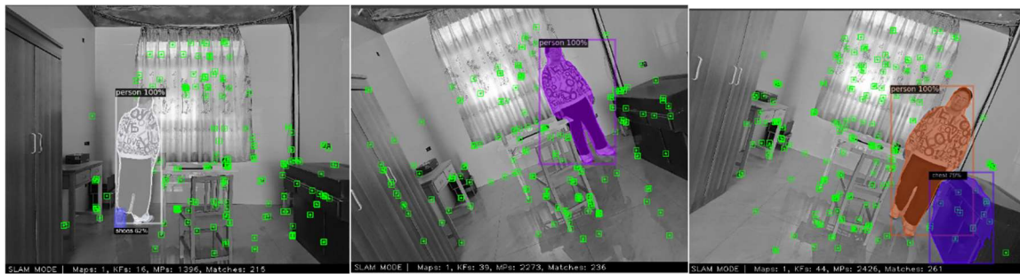
(c) Image after filtering out dynamic feature points
