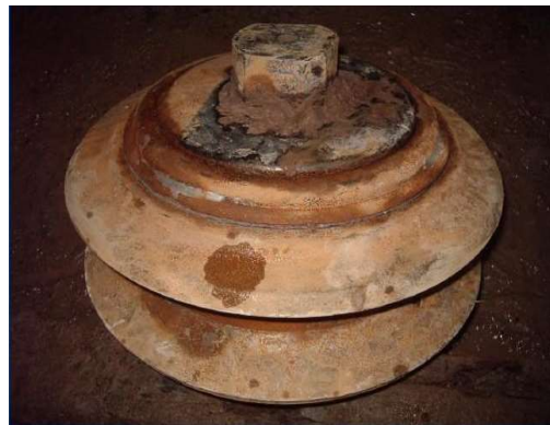
Fig.3 Photos of tool wear
