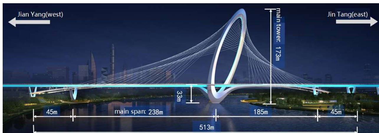
Fig. 1 The elevation arrangement of Tuojiang Bridge
