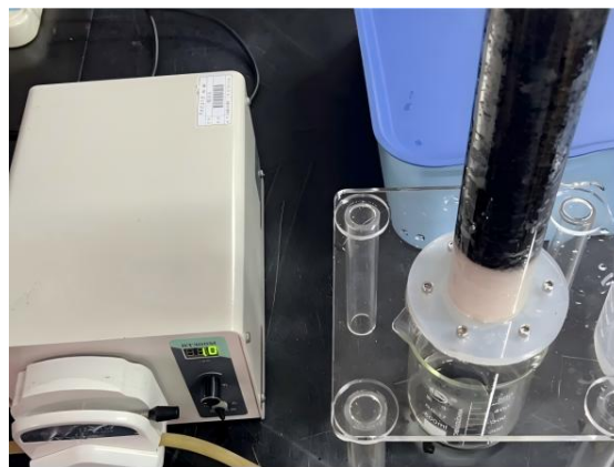
Figure 1. Dynamic column leaching apparatus used in this study
