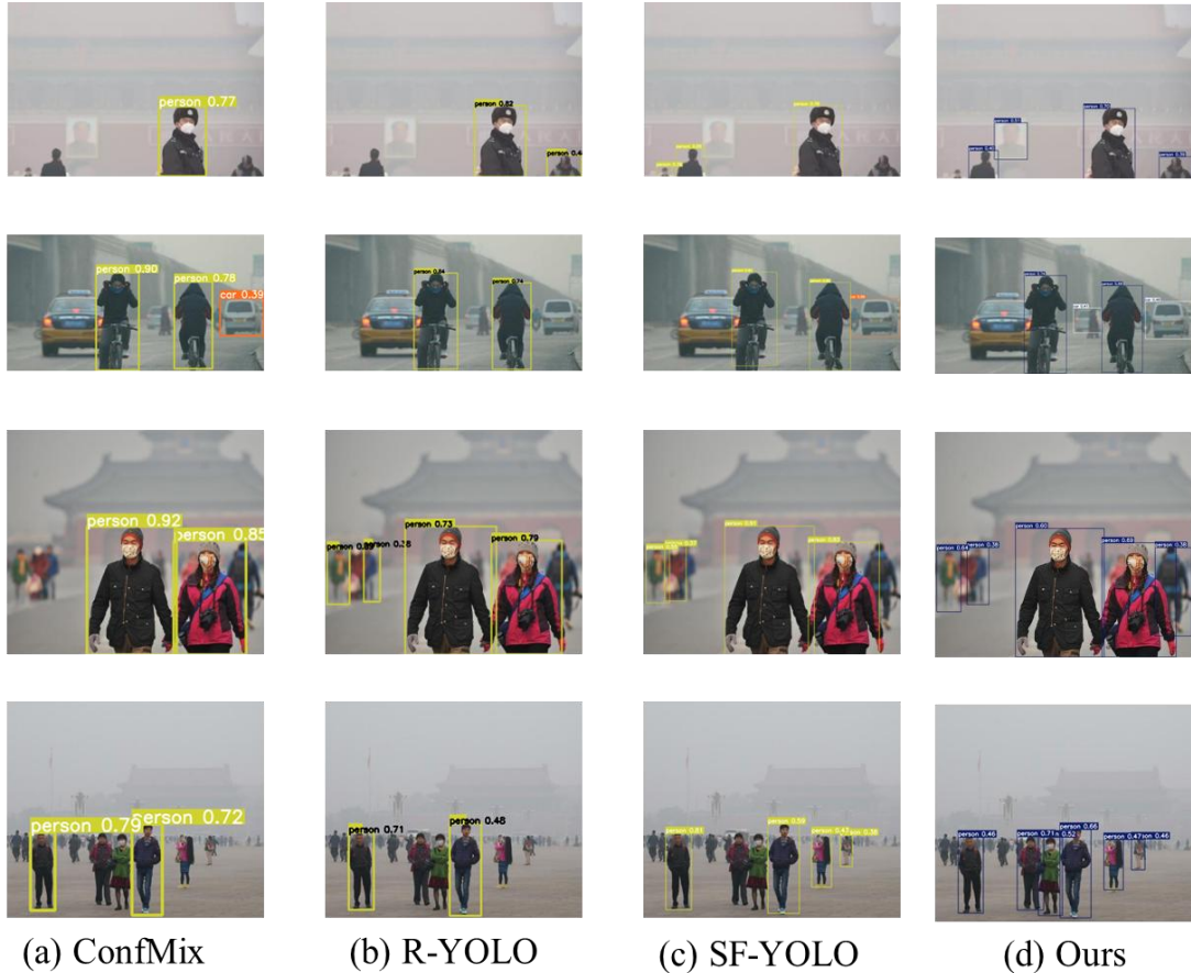
Figure 5. Visualization of Detection Results on Real-World Foggy Scenes
