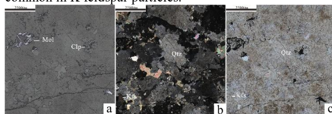
a-the characteristics of a-nonmetallic minerals under single polarization; b-nonmetallic mineral characteristics under orthogonal polarized light; characteristics of c-metallic minerals under reflected light Qtz-quartz; Kfs-potassium feldspar; mol-molybdenite; clp-chalcopryite
